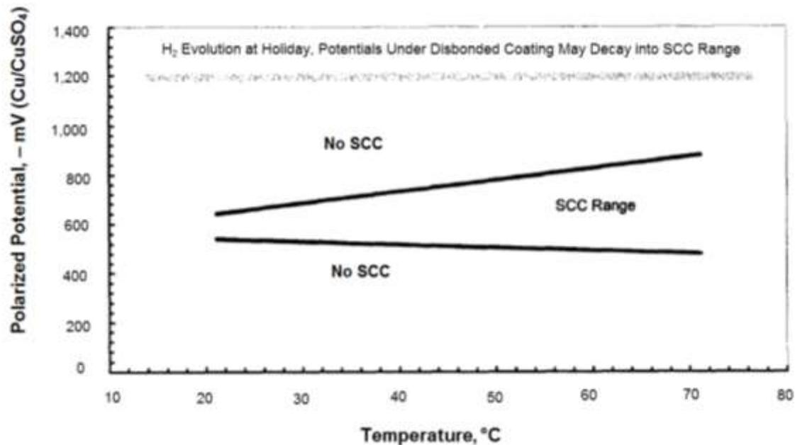
**Figure 2: SCC Range of Pipe Steel in Carbonate/Bicarbonate Environments.<sup>72</sup> Note: This figure is not applicable to all grades of steel and in all electrolytes. (For conversion, °F = 9/5 °C + 32).**
