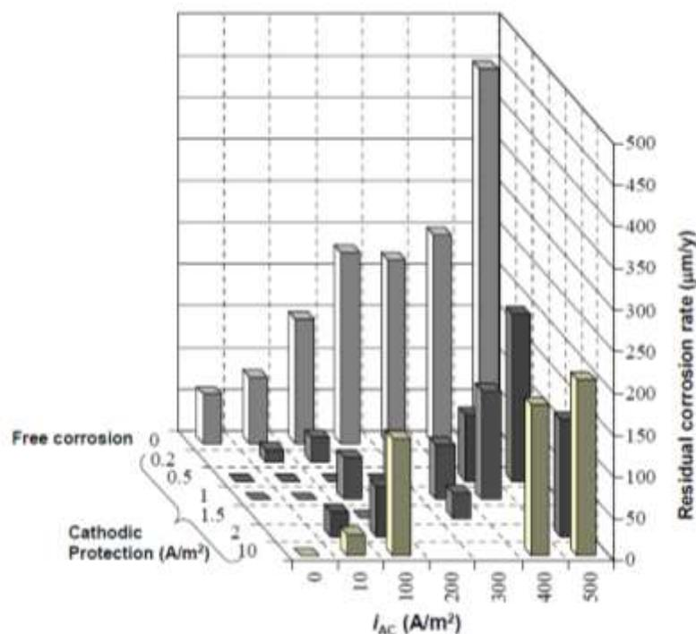
**Figure 1: Residual Corrosion Rate of Carbon Steel Specimens as a Function of AC and CP Current Density. Laboratory Tests Performed in Simulated Soil Conditions.<sup>70</sup>**
